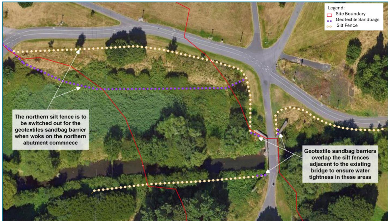
Figure 10-3: Location of Silt Fences and Geotextile Sandbags Adjacent to River Tolka
